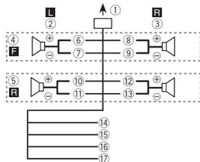
Perform these connections when using a subwoofer without the optional amplifier.
